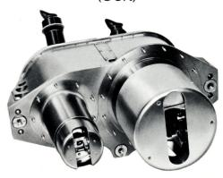
The OUA, a sextant-telescope package, is used to sight on known reference stars and landmarks for the fine angle measurements needed in navigational checks. In most operations, the Command Module pilot will use the telescope to locate a target star, then sight the selected star in the magnified field of view of the sextant to make precise measurements.
