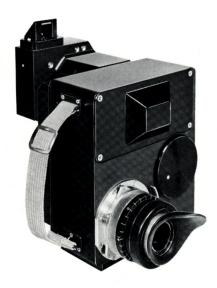
The rangefinder will provide the Command Module pilot with a reading of the distance to the Lunar Module during the rendezvous maneuver.
