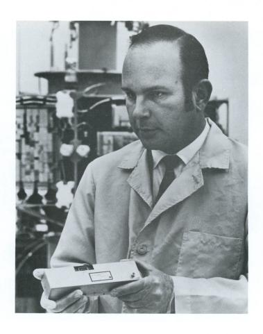
Philco-Ford employe holds small transmitter that sends scientific information from the moon to receiving stations here on earth. The small package is the transmitter for the Apollo Lunar Surface Experiments Package (ALSEP), which is left behind on the moon by astronauts to gather scientific information. The transmitter was designed and built by Philco-Ford Corporation.
